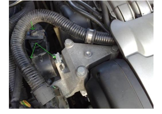
Once these bolts are removed, the stabilizer arm can be taken out easily, which then gains access to the top of the mount.
