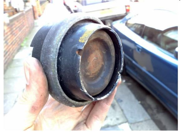
Now the engine mount has been removed you will be left with the bottom of the old mount still attached to the car. Hopefully this will be easy to just remove by twisting the remains out, as its actually the bottom bolt still attached, but mine was a b\*tch and wouldnt come out, so I welded a bolt to the middle of the remains and then just used a ratchet to
