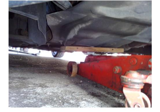
Once, The engine has been jacked up and is firmly secure, its time to start removing the bolts to gain access and move the engine mount. Firstly you need to use a size 20 torx bit to remove the screw holding the ECU wiring.
