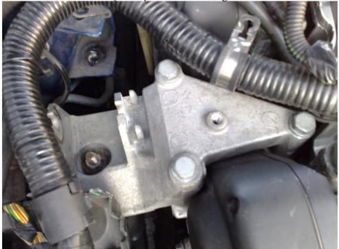
Now refit the stabilizer arm and replace/tighten the bolt which goes downwards on the windscreen end and the bolt which goes horizontal through the other end (I found it easier slot the horizontal bolt through rubber end before you refit the stabilizer arm, this is because the bolt is so long, it isnt possible to slot the bolt through once the stabilizer arm is refitted unless you remove the ECU box, which is unnecessary)
