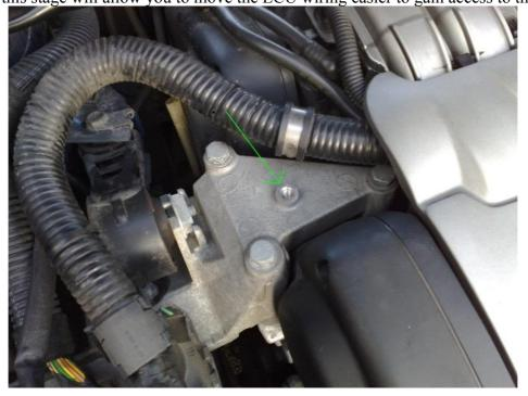
Now you need to remove the stabilizer arm. This is done by removing the single bolt nearest to the windscreen, and then the bolts which slots through the front of the stabilizer arm. All the bolts will be size 16 metric (well they were on mine) You should inspect the stabilizer arm for wear in the rubber sections as this may need to be replaced also (in my case the small rubber end has worn a little so I will be replacing that soon)
